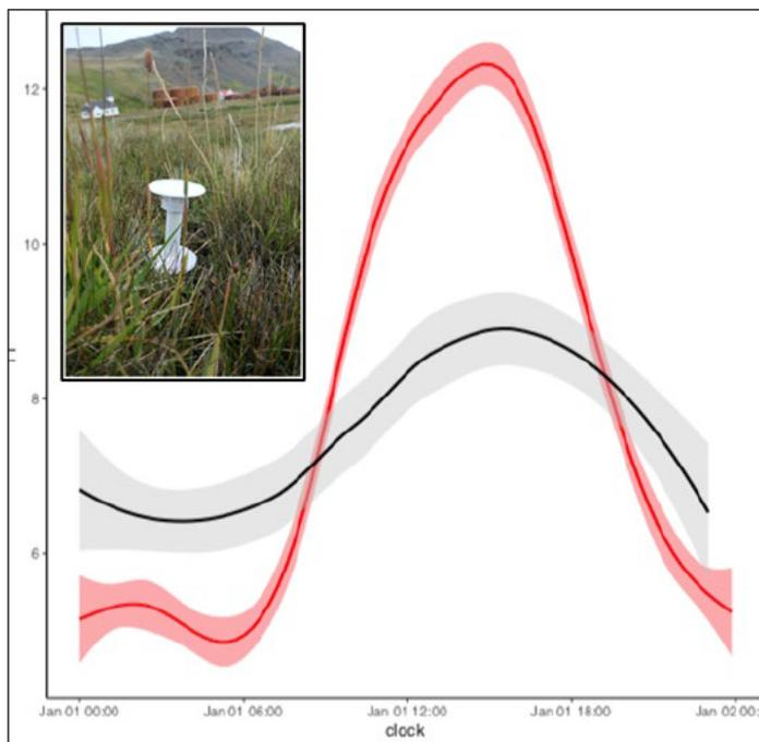
**Figure 8.** Inset: One of the TOMST (TMS-4) data-loggers placed in the field in South Georgia, to capture the temperature regime experienced by plants at the plant level. Plot: average temperature (°C) and 95% confidence envelope, over a 24-hour cycle captured ~15 cm aboveground with a TOMST data logger (red) and 1 m aboveground at KEP weather station (black).
